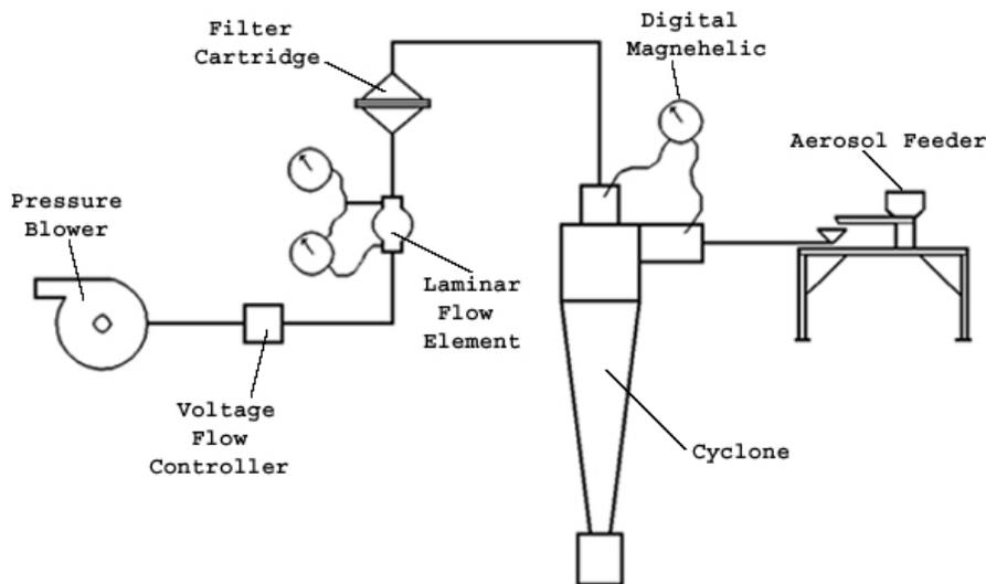
Figure 2. Cyclone testing system.
