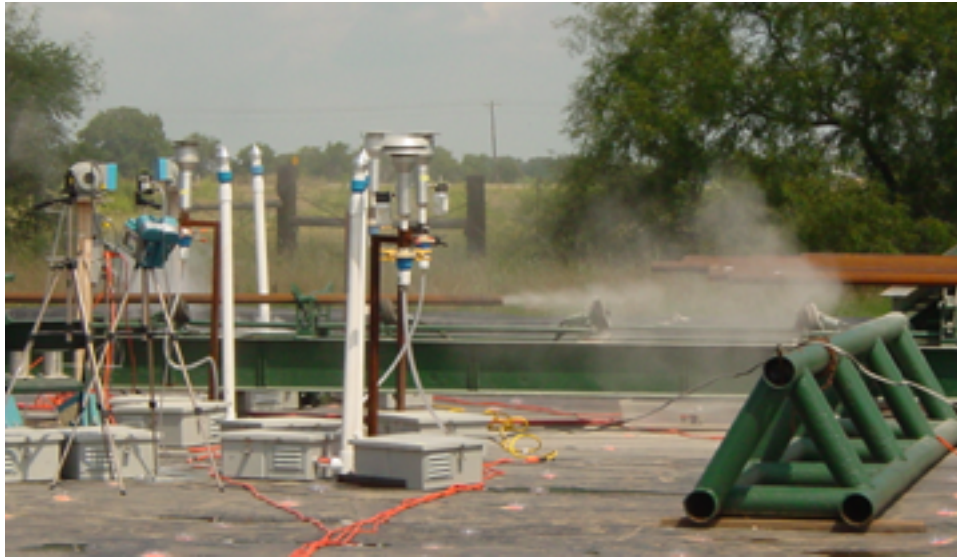
Figure 8. View of PM plume from oil pipe.
