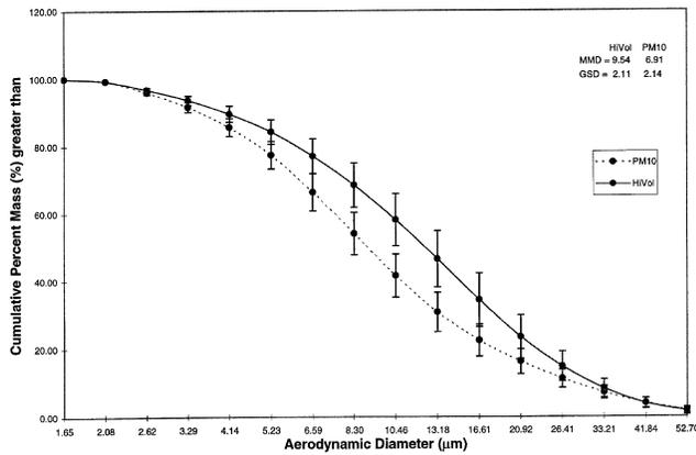
**Figure 1—Mass fraction of feedlot dust of given size captured with high volume and PM<sub>10</sub> samplers.**
