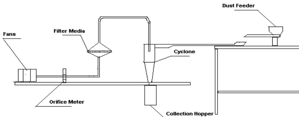
Figure 4. Schematic of the system used for cyclone testing
