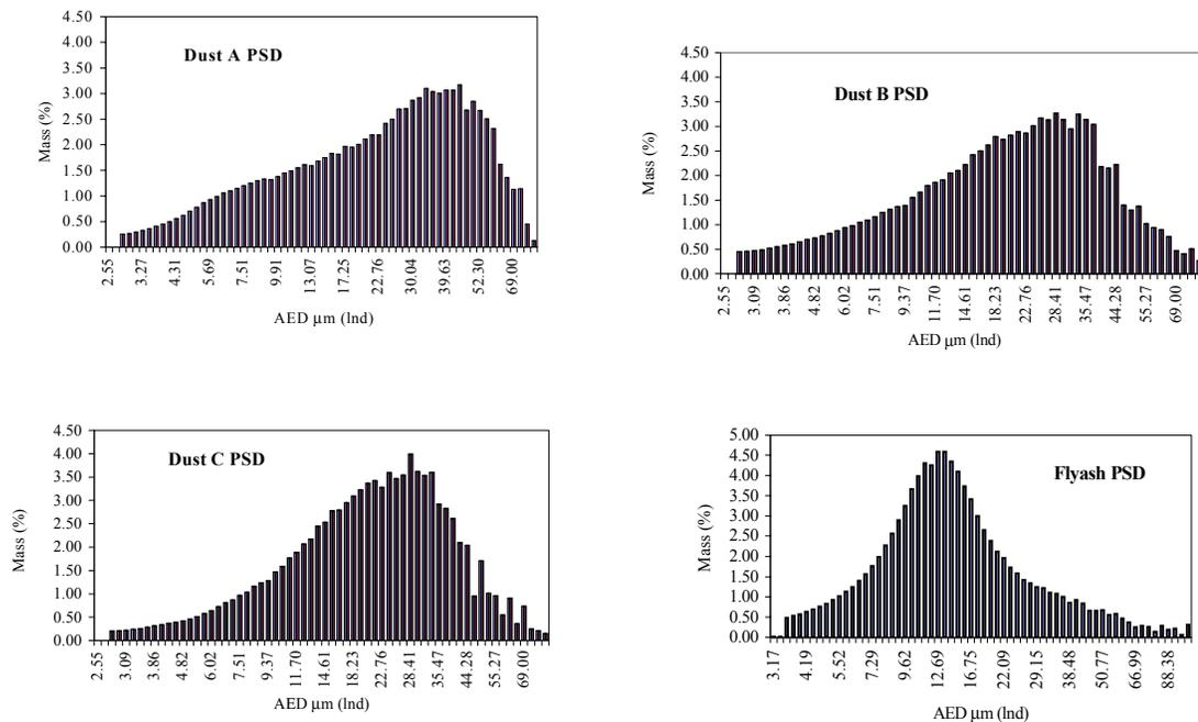
Figure 3. Particle size distributions of fine dust in trash A, B, C and fly ash PSD
