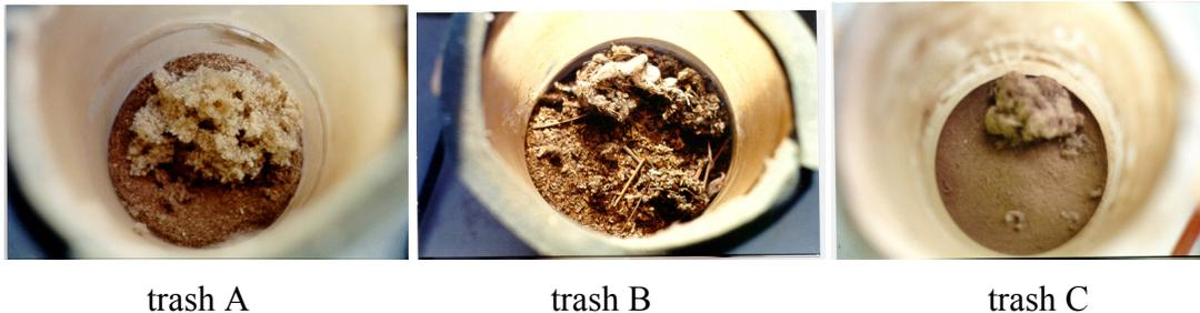
Figure 2. Gin trash collected by the cyclone
