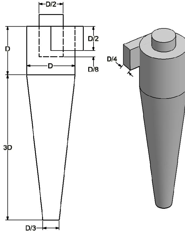
Figure 1. 1D3D cyclone configuration.
