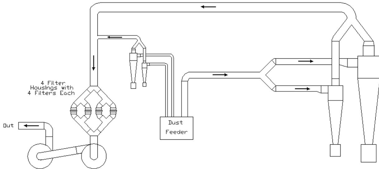
Figure 2. Cyclone testing system.
