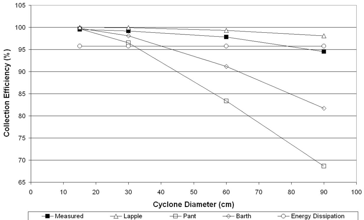
Figure 6. Modeled versus measured collection efficiencies.
