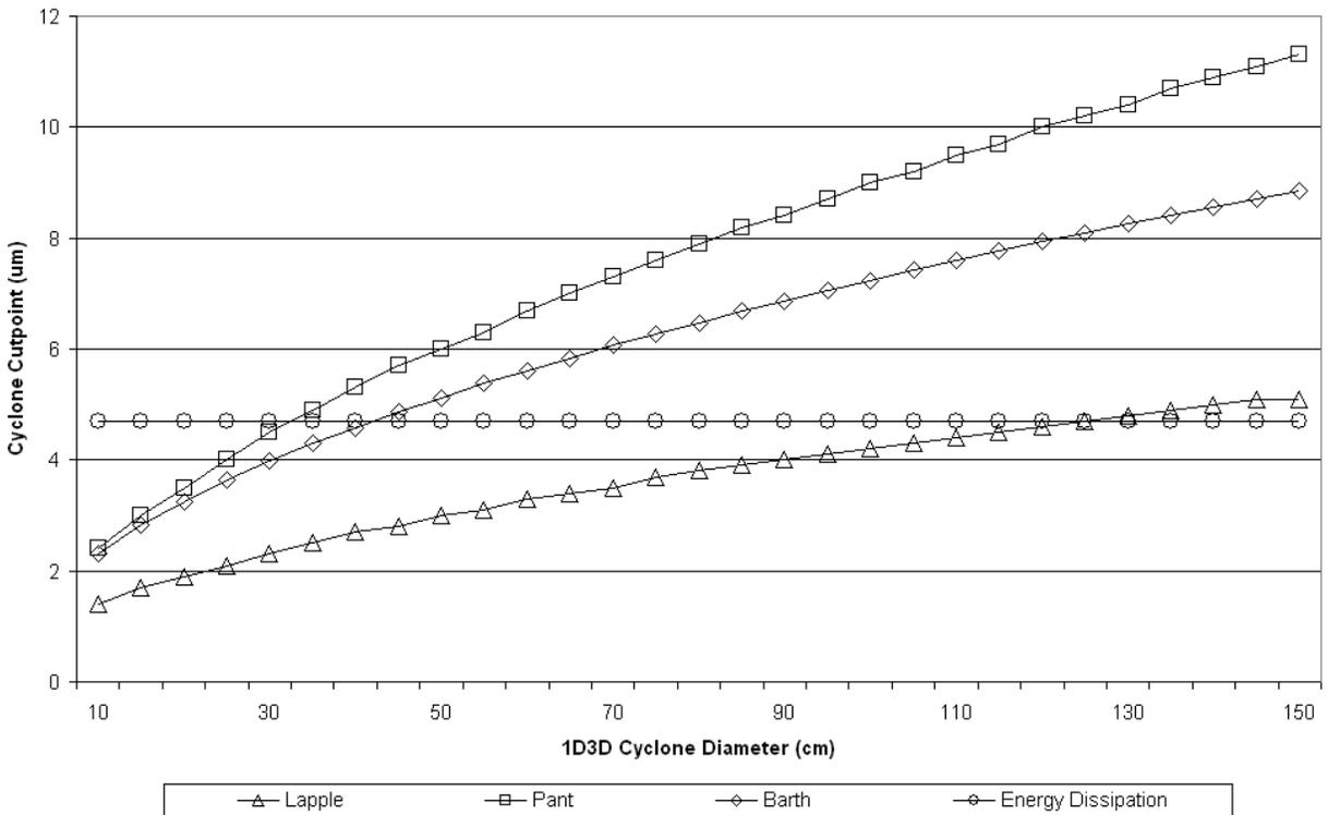
Figure 4. 1D3D cyclone cut point models.
