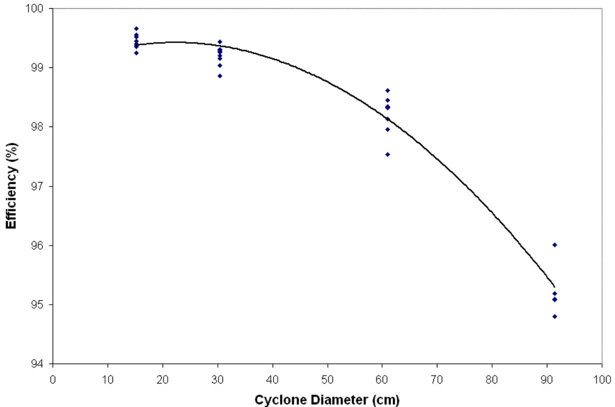
Figure 5. Regression of collection efficiency versus cyclone diameter for conditions tested.
