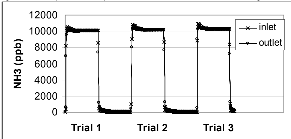
Figure 8. Adsorption – desorption curves of NH 3 on 46 m Teflon Tubing at
