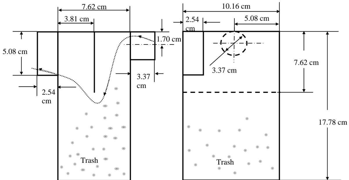
Figure 2. Baffle type pre-separator design and dimensions
