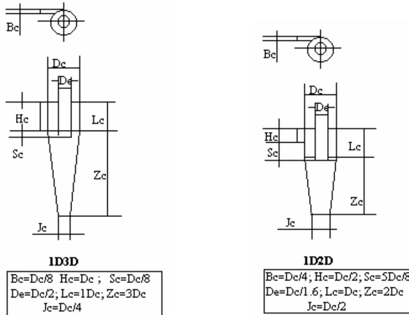
Figure 3. Cyclone designs and dimensions
