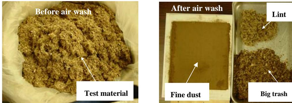
Figure 4. Gin trash: before and after air wash
