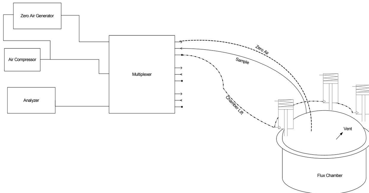
Figure 1. Multiplexed chamber setup.
