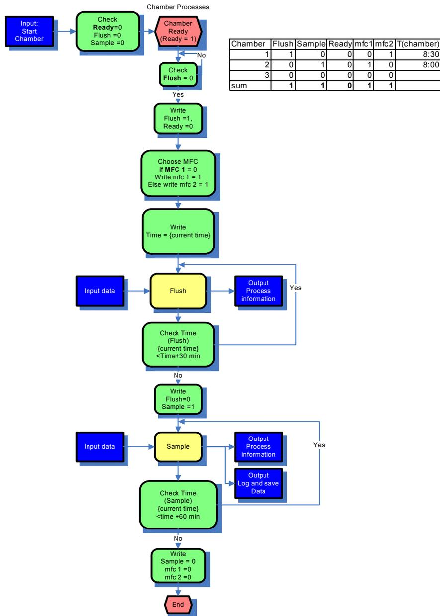
Figure 3. Multiplexer process diagram.
