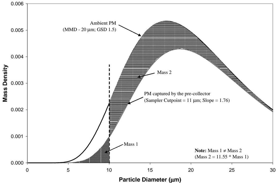
**Figure 3.** PM<sub>10</sub> stack sampler nominal cut (sampler d<sub>50</sub> = 11 μm; slope = 1.76) for a lognormal PSD with a MMD = 20 μm and GSD = 1.5.
