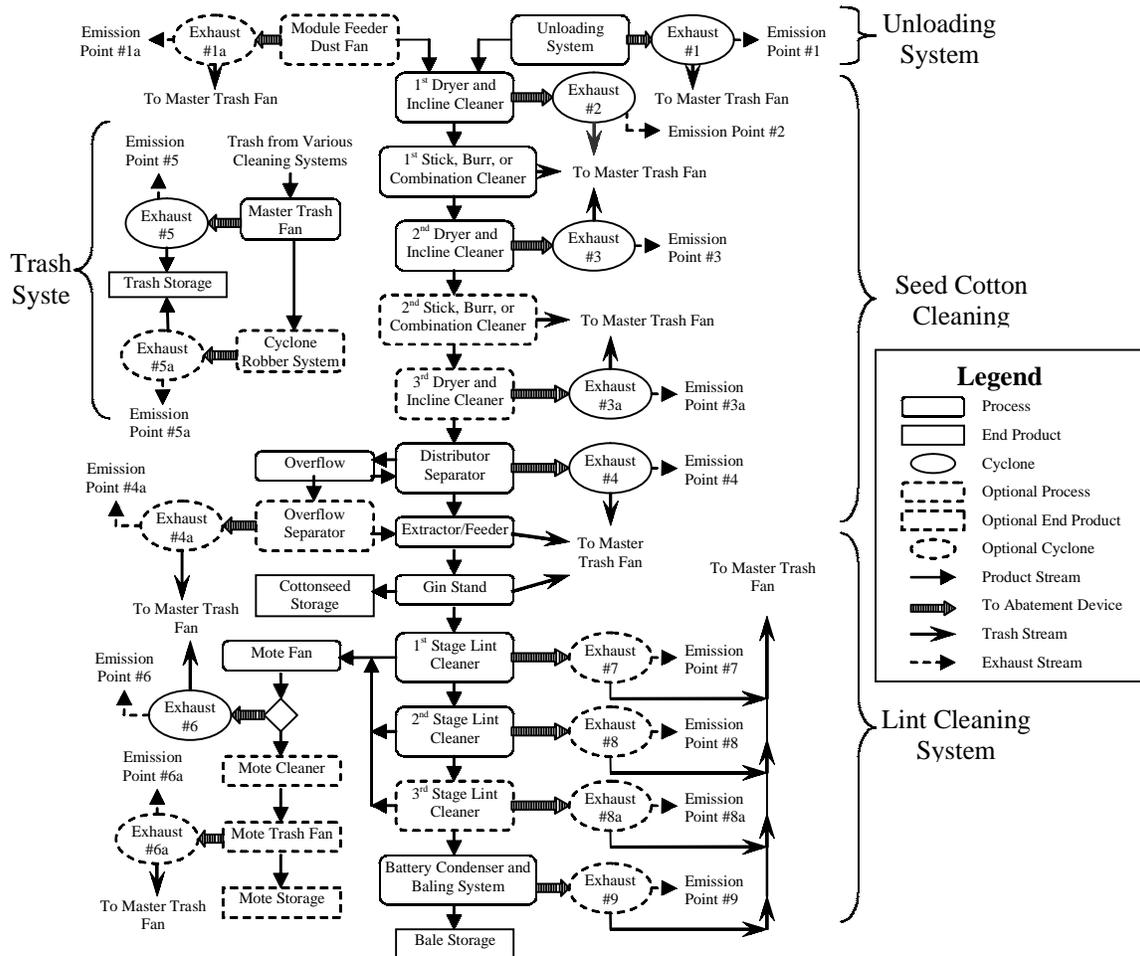
Figure 4. Cotton Gin Material Handling System Flow Diagram.
