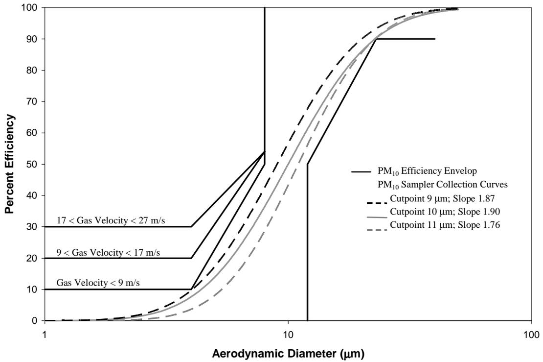
Figure 1. Method 201a PM<sub>10</sub> cyclone efficiency envelope and theoretical PM<sub>10</sub> cyclone collection efficiency curves.
