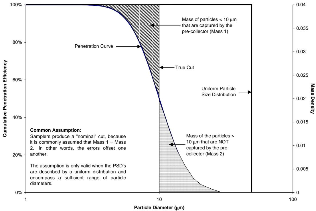
Figure 2. PM<sub>10</sub> sampler nominal cut for a uniform PSD.
