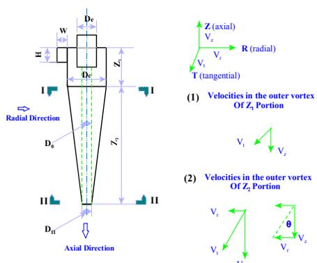
Figure 3. Cyclone dimensions and the velocity distributions
