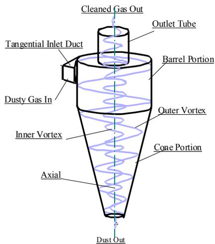
Figure 1. Schematic flow diagram of a cyclone
