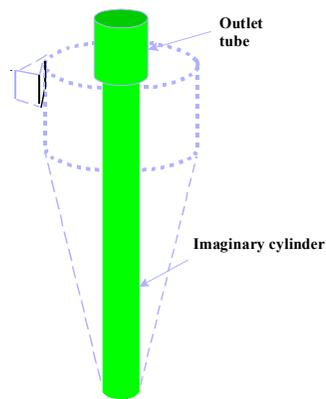
Figure 6. The imaginary inner vortex cylinder
