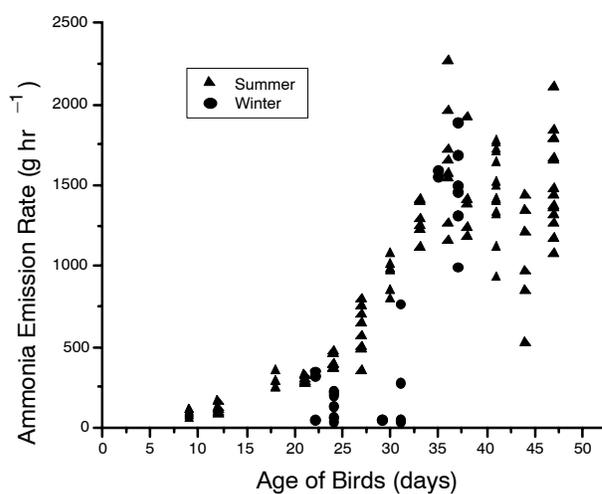
**Figure 8. Ammonia emission rate (g hr<sup>-1</sup>) per building (27,500 birds) versus age of birds (days) measured in four commercial tunnel-ventilated broiler houses in central Texas during June–December 2000.**
