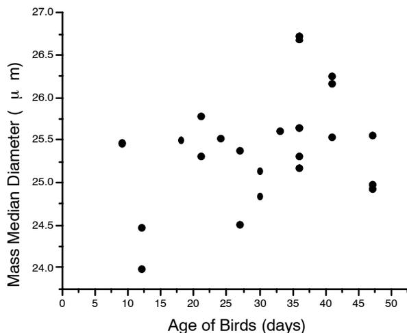
Figure 4. Mass median diameter of particulate matter ( $\mu\text{m}$ ) versus age of birds (days) for particulate matter sampled in commercial tunnel-ventilated broiler houses in central Texas during June–December 2000.
