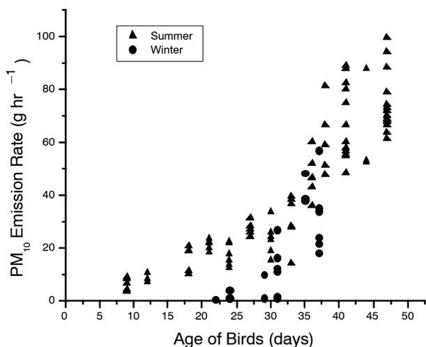
**Figure 7. PM<sub>10</sub> emission rate (g hr<sup>-1</sup>) per building (27,500 birds) versus age of the birds (days) measured in four commercial tunnel-ventilated broiler houses in central Texas during June–December 2000.**
