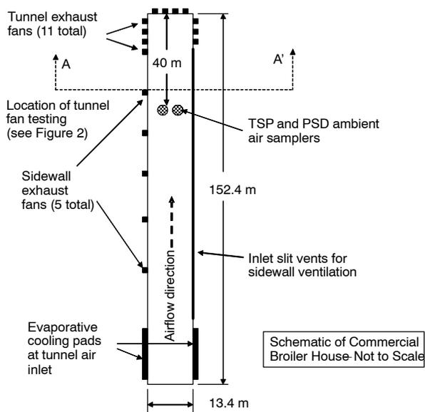
Figure 1. Schematic of the plan view of commercial boiler houses used in the study showing the location of the air samplers and ventilation fans.
