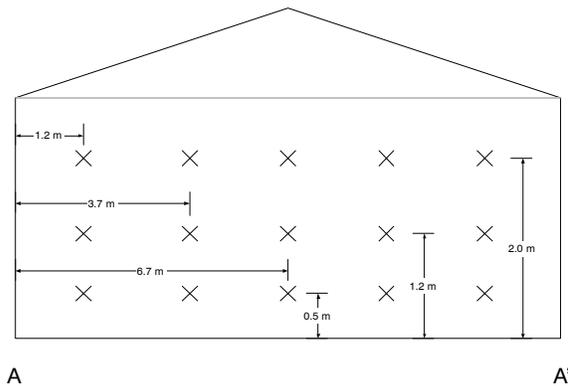
**Figure 2. Sampling positions for measurement of ventilation rates during tunnel ventilation of commercial broiler houses. Each "x" marks a location where the air velocity was recorded. The ventilation rate for a given set of operating fans was calculated from the mean air velocity at the 15 points times the cross-sectional area of the building.**
