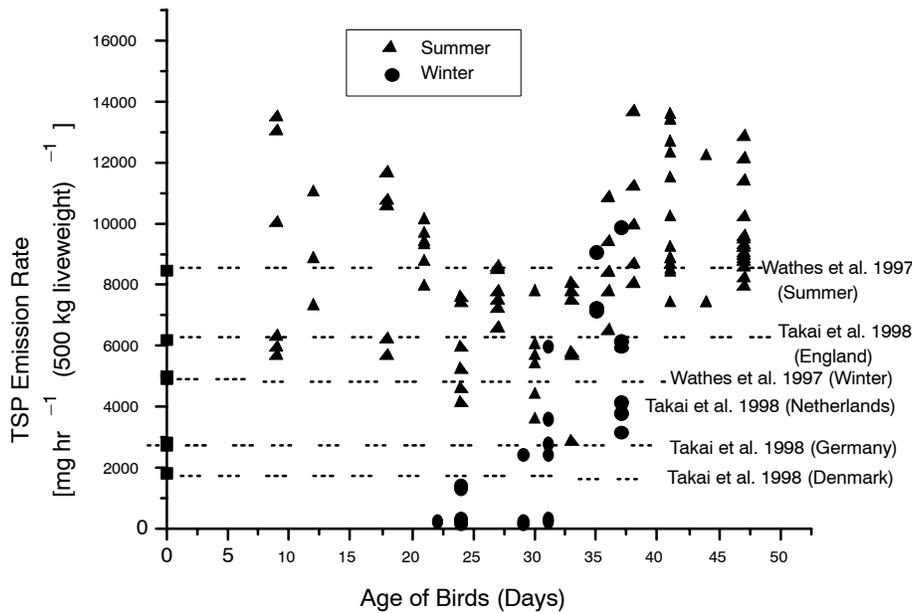
Figure 9. Calculated emissions of total suspended particulates ( $\text{mg hr}^{-1} 500 \text{ kg}^{-1}$ ) versus age of the birds (days) measured in four commercial tunnel-ventilated broiler houses in central Texas during June–December 2000 compared to concentrations reported in the literature.
