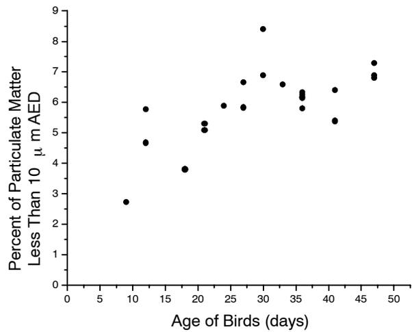
Figure 5. Mass percentage of particulate matter classified as  $\text{PM}_{10}$  versus age of birds (days) determined from particle size distributions calculated with a Coulter Counter Multisizer and sampled in four tunnel-ventilated commercial broiler houses in central Texas during June–December 2000.
