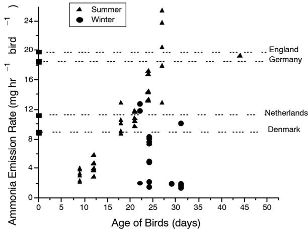
Figure 10. Ammonia emission rates ( $\text{mg hr}^{-1} \text{bird}^{-1}$ ) versus age of the birds (days) measured in four commercial tunnel-ventilated broiler houses in central Texas during June–December 2000 compared to mean emission rates (represented by dotted lines) reported by Groot Koerkamp et al. (1998).
