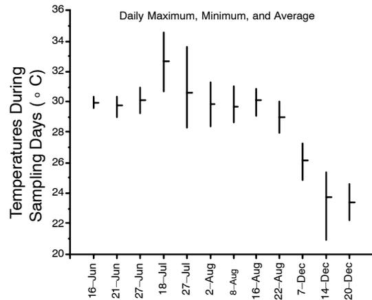
Figure 11. Dry-bulb temperature during sampling periods in four commercial tunnel-ventilated broiler houses in central Texas, showing maximum, minimum, and mean values. Samples were taken every 12 seconds during PM sampling, for approximately 10,000 data points per day.
