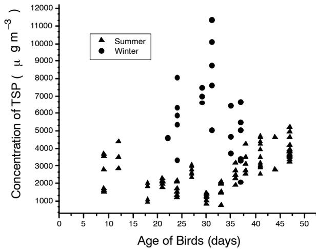
Figure 3. Concentration of total suspended particulate matter ( $\mu\text{g m}^{-3}$ ) versus age of birds (days) measured in four commercial tunnel-ventilated broiler houses in central Texas during June–December 2000.
